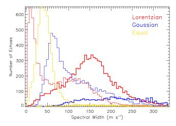
**Fig. 3.** A set of histograms showing the number of echoes found within  $5 \,\mathrm{m\,s^{-1}}$  bins of spectral width on beam 4 during the interval, 12:15 to 15:00 UT on 10 December 1999. The results have been sorted according to spectral fit type: Lorentzian fit (red), indeterminate fit (yellow), and Gaussian fit (blue); and into categories above (bold) and below (thin) the SWB.
