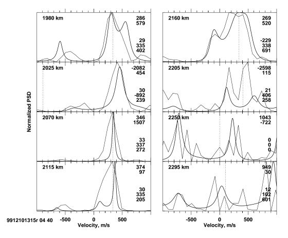
**Fig. 5.** Eight examples of DFT Doppler spectra (light curves) and Burg spectra (bold curves) calculated using ACFs recorded on beam 4 between ranges 1980 km and 2295 km at 13:15 UT on 10 December 1999. In each panel, the Doppler velocities of the two main peaks are given at top right, and the FITACF power, line-of-sight velocity, and spectral width are given at bottom right. The spectra at all ranges except 2025, 2070, and 2115 km are double-peaked spectra using our selection criteria.
